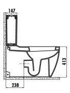
There is only hidden connection for the self cleaning pipe&internal mechanism. Not suitable for side connection.
